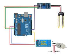
Fig 2: Circuit diagram of water dispenser
